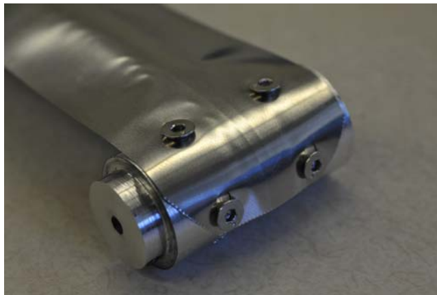
Figure 3: Boom is Secured to Drum
