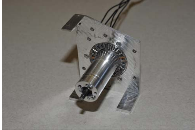
Figure 4: Sleeve Attaches To Motor for Later Mounting
