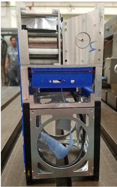
Figure 4. Prototype of DMD with CubeSat structure.
