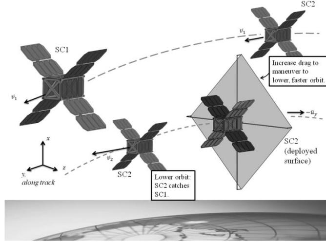
**Figure 1. Conceptual sketch explaining differential drag control. Spacecraft 2 increases its drag, thus lowering its orbit and increasing its speed, to catch up with spacecraft 1 in terms of orbital polar angle.**
