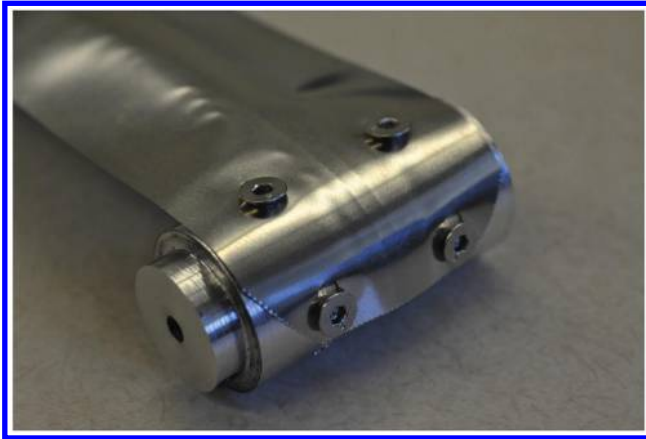
Fig. 3 Boom secured to drum.
