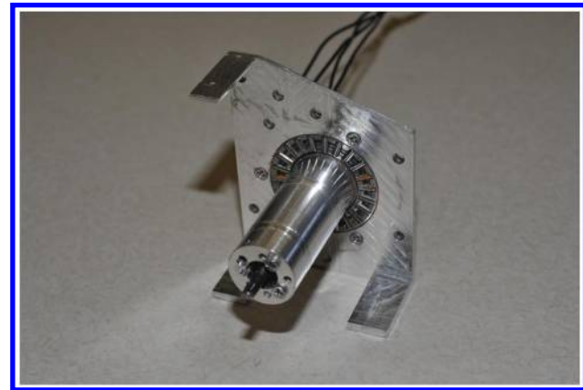
Fig. 4 Sleeve attached to motor for later mounting.
