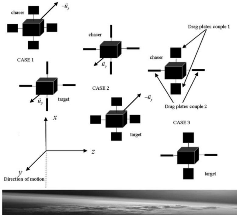
**Figure 1. Drag panels concept to generate differential drag (obtained from 5).**
