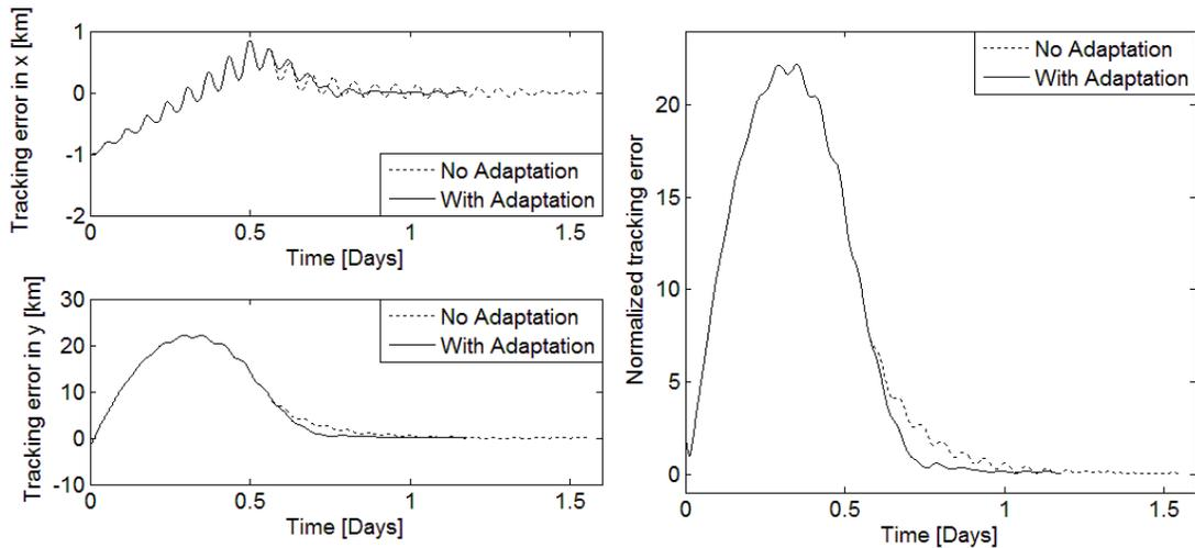
**Figure 7. Numerical simulation result error over the entire maneuver: (Left top) x error, (Left bottom) y error, (Right) Normalized error.**
