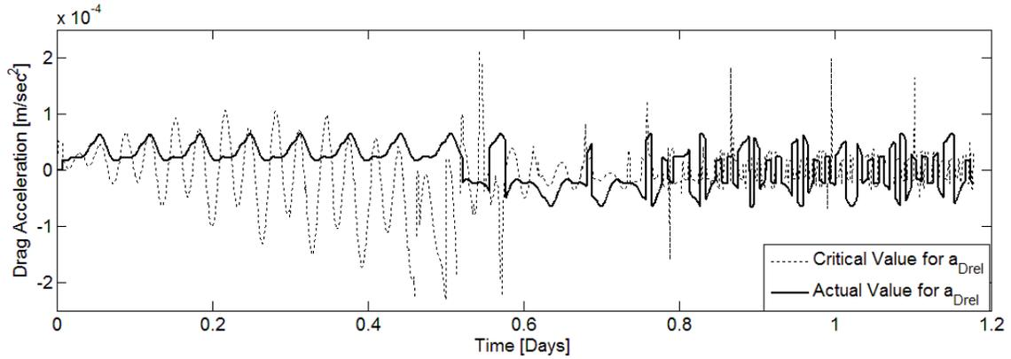
**Figure 6. Numerical simulation result: Comparison between the critical value for the magnitude of the differential acceleration ( $a_{Dcrit}$ ) and the actual value of the differential acceleration for the adaptive controller.**
