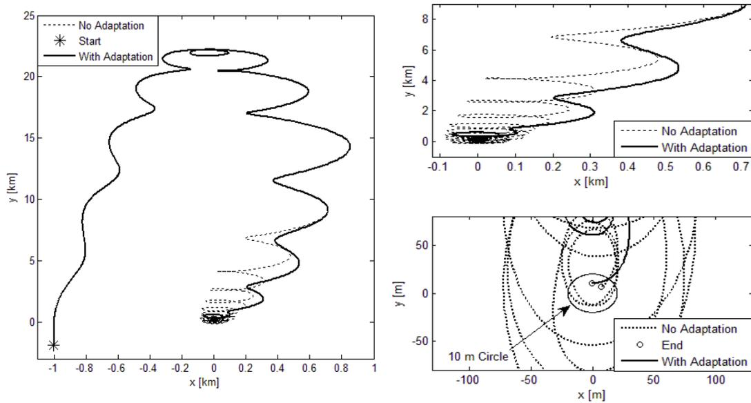
**Figure 3. Numerical simulation result maneuver trajectory in the x-y plane: (Left) Complete maneuver, (Right top, and bottom) Final Stages of the maneuver.**
