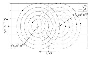
Figure 5.2: Qualitative shape of the curves on the phase plane of the harmonic oscillator subsystem  $(z_3 \text{ vs. } z_4)$  in case of constant thrust along the y axis for both the Hill-Clohessy-Wiltshire and the Schweighart-Sedwick models.
