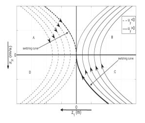
Figure 5.1: Qualitative shape of the curves on the phase plane of the double integrator subsystem  $(z_1 \text{ vs. } z_2)$  in case of constant thrust along the y axis for both the Hill-Clohessy-Wiltshire and the Schweighart-Sedwick models.
